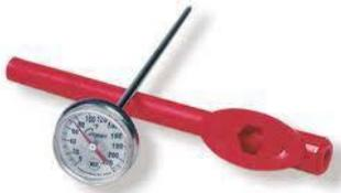
A metal-stemmed thermometer ranging from 0-220°F for checking hot and cold food is required. It must read in 2°F increments, cannot be glass, and must be calibrated prior to the event.
